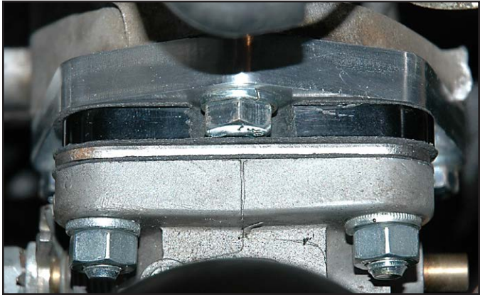
Photo from the top of the adapter showing all the parts installed, with the carburetor fully mounted.
